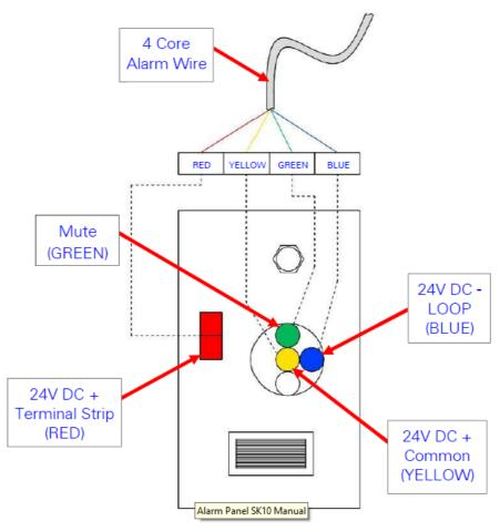
Alarm Panel Wiring Diagram
